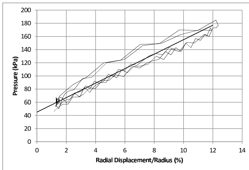
Figure 4.10: Air Membrane Calibration Test With Fitted Slope for Data Correction
